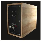
The Rebel2 is a two-way, stand-mounted, reflex-loaded design, utilizing a 20mm soft ferro-fluid textile dome tweeter and a specially treated 120mm midrange/bass unit. Penaudio only uses soft, non-resonant tweeter units in their speakers. The Rebel2 frequency range is noted in both anechoic response (80-2200Hz) and in room (50-20000Hz) with a quite high crossover at 4000Hz.
